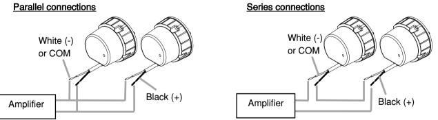
• To avoid amplifier failure, do not simultaneously connect both low- and high- impedance speakers to the amplifier. Ensure that only one type is connected.
