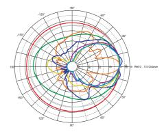
NOTES: Frequency response measured at 4m (13.12ft). For better detail, only light smoothing (1/12th octave) has been used. Polars were acquired by placing the unit on a computer controlled turntable inside a 411 m³ (14514 ft³) anechoic chamber. Measurement distance is 4m (13.12ft).
