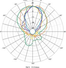
NOTES. 1.Frequency response: referred to 1 m; low end obtained through the use of near field techniques; one-third octave smoothed for correlation with human hearing. 5.Polars were acquired by placing the unit on a computer controlled turntable inside our anechoic chamber. Measurement distance was 4 m.
