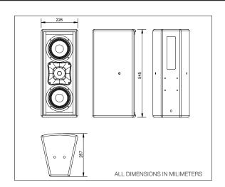
The DAS WR-8826 is a two-way loudspeaker system for applications covering speech reinforcement, program reproduction and live music productions specially designed to be used outdoors due to its specific treatments against dust, water and humidity.
