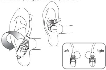
Remove the sleeves from the earphone before cleaning the wax. Smoothly insert the wax removal loop into the nozzle, and peel off the wax inside. Be careful not to damage the internal earphone sound filter when cleaning.
