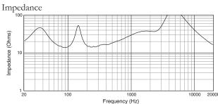
Measurements obtained in full passive crossover mode with no signal processing. Graphs are from unaltered measured data.
