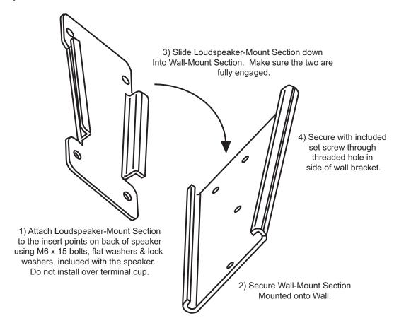
**IMPORTANT:** Brackets **MUST** be installed by qualified personnel in accordance with safe installation practices.
