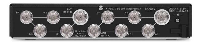
The ASA 214 active antenna splitter is built in a full metal housing and ships with 8 BNC cables included. The splitter runs up to 4 receivers of the ew series with two antennas. The UHF-Version includes the NT 1-1 power supply with EU, UK and US adapters, while the ASA 214-1G8 includes the NT 1-1 with EU, UK and AU adapters.
