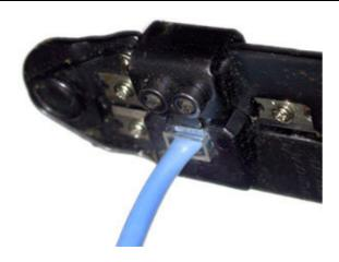
Note: Diagram A, The cable do not go all the way to end of the connector
