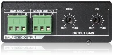
EMPR-8007 provided 2 balanced outputs. BGM audio signal output just from background music inputs choose by user and it used in uninterrupted system. Where our MIXED audio signal output are combination from the signal of our EMKP-8001 digital paging console and background music source which normally we called it as interrupted system. Both of the audio signal outputs have individual gain control.
