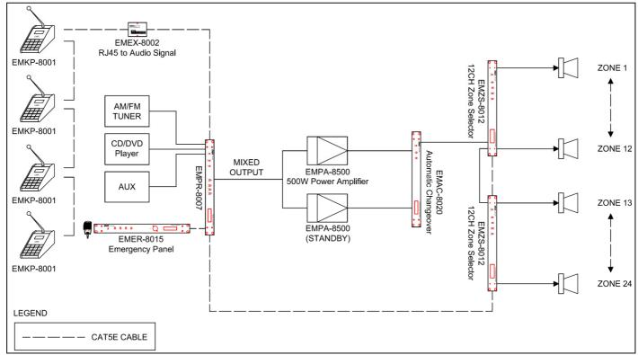
**Diagram 1.0:-** Single Line diagram for Interrupted System Configuration
