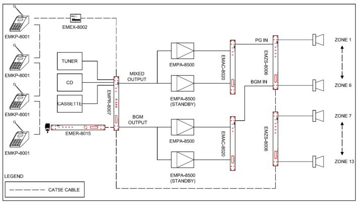
**Diagram 1.1:-** Single line diagram for Uninterrupted System Configuration
