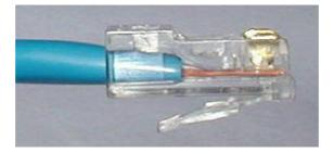
6. Check the color orientation, check that the crimped connection is not about to come apart, and check to see if the wires are flat against the front of the plug. If even one of these is incorrect, you will have to start over.
