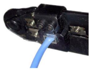
The cable do not go all the way to end of the connector
