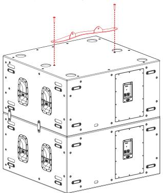
Next, place the 2 x ES-158, and screw them to the AX-SF2158 using the rear panel M10 screws of the ES-158
