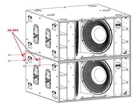
Next step, screw the AX-SF2158 to the top subwoofer using the M 10 screws
