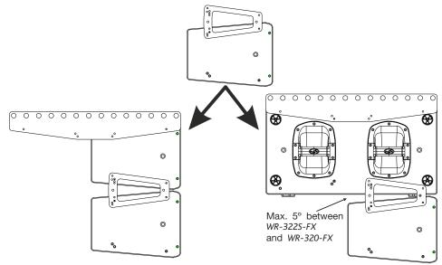
As an example we will mount the following array: 1x WR-322S-FX + 4x WR-320-FX, with angles: 0°, 0,5°, 1° and 5°.
