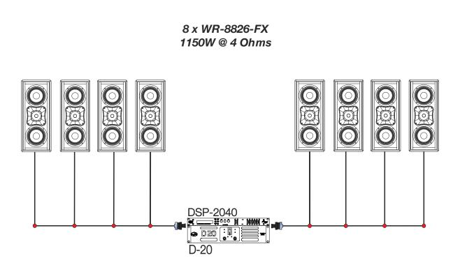
Four WR-8826-FX (16ohms each) in parallel mode per channel. Refer to the user manual of the D-20 amplifier for SPEAKON connection.
