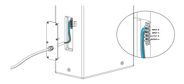
3.- Fix the cover of the rear part of the enclosure with six screws.
