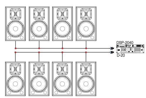
8 x WR-6412-FX (or WR-6415-FX) 2100W @ 2 Ohms
