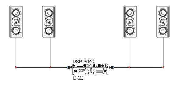
Two WR-8826-FX (16ohms each) in parallel mode per channel. Refer to the user manual of the D-20 amplifier for SPEAKON connection.
