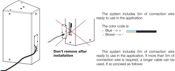
1.- Prepare the rear part of the enclosure for cable connection, removing the existing cable.
