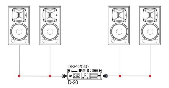
Two WR-6412-FX or WR-6415-FX (8 ohms each) in parallel per channel. Refer to the user manual of the D-20 amplifier for SPEAKON connection.
