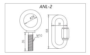
Each ANL-2 eyebolt has a rated working load of 200 kg. (440 lb). Each ANL-2 carabiner has a working load of 330 kg (726 lb). If using other hardware, make sure it is rated to handle the required load.
