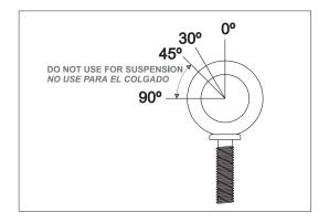
The following illustrations show different views on eyebolt flying for a single box. The length of the back cables or chains determines the vertical angle of the box.
