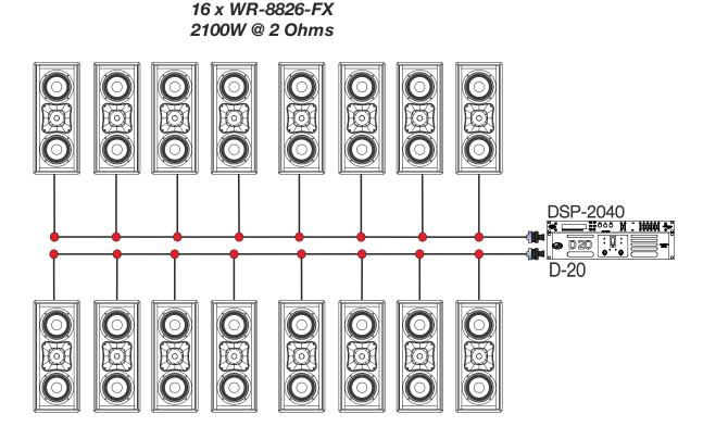
Eight WR-8826-FX (16ohms each) in parallel per channel. Refer to the user manual of the D-20 amplifier for SPEAKON connection.
