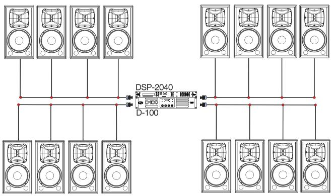
Four WR-6412-FX or WR-6415-FX (8 ohms each) in parallel per channel Refer to the user manual of the D-100 amplifier for SPEAKON connection.
