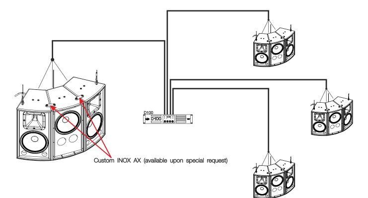
2 tops and 1 sub are ideal to be used with one amplifier channel (using the subwoofer's selector in the "PASSIVE SYSTEM" position).
