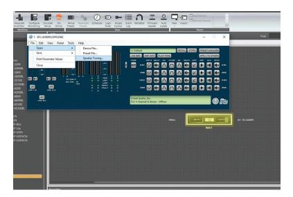
**Important**: Note that since it is an FIR filter you will not see filters above 300Hz as they don't manifest themselves the same way an IIR filter would in that setting. However, they will be engaged. In addition, you will have plenty of filters and delays to make suitable on-site adjustments.
