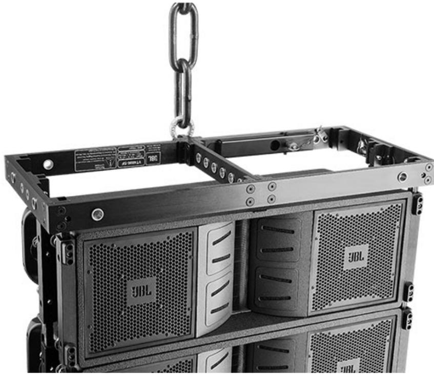
Figure 3: Single point suspension using VT4886-SF short frame hole number 7.
