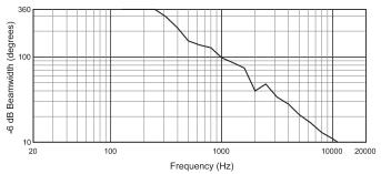
Vertical Beamwidth, Single Line Array Element
