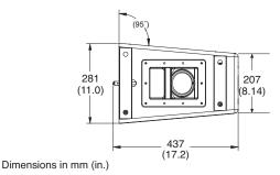
System Dimensions (WxHxD): 787 mm x 281 mm x 415 mm including attached suspension hardware
