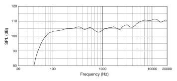
Frequency Response, On-Axis, Single Line Array Element
