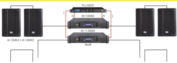
SUB-118B Compatible for 1 unit or 2 unit of rX-12MK2 / rX-15MK2 each side.
